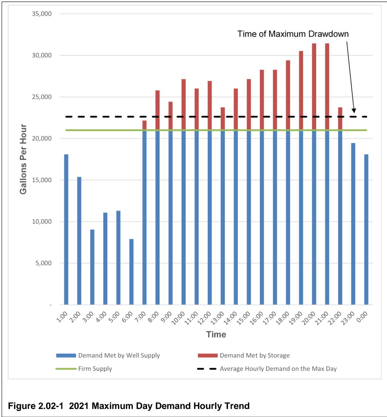
Table 2.02-1 shows the results of the maximum day in 2021. The utility is currently in need of additional supply but has adequate storage to meet peak hourly demands on the maximum day. Since the current maximum day demand exceeds the firm supply capacity, the system is currently vulnerable to storage depletion if multiple maximum days were to occur in a row and a well or booster pump were out of service.
