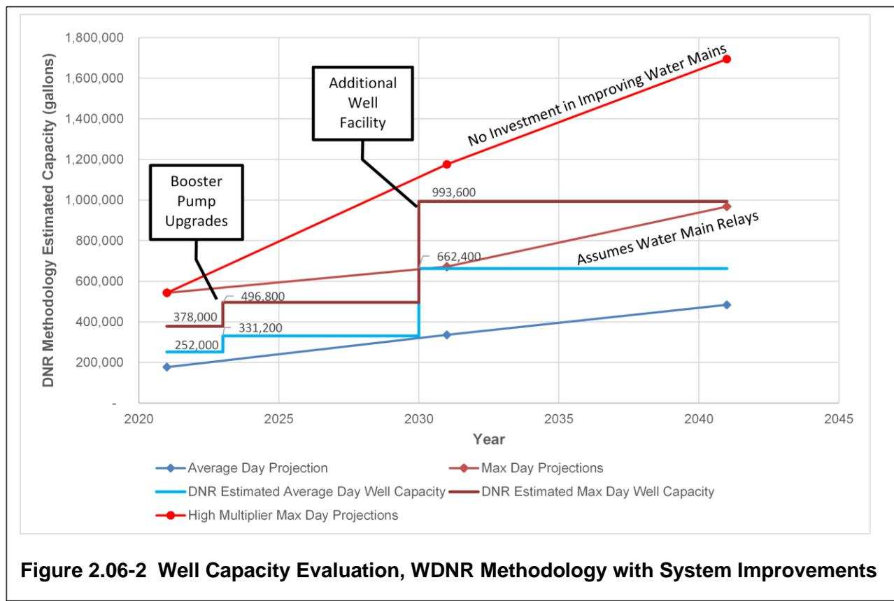
Figure 2.06-2 Well Capacity Evaluation, WDNR Methodology with System Improvements
